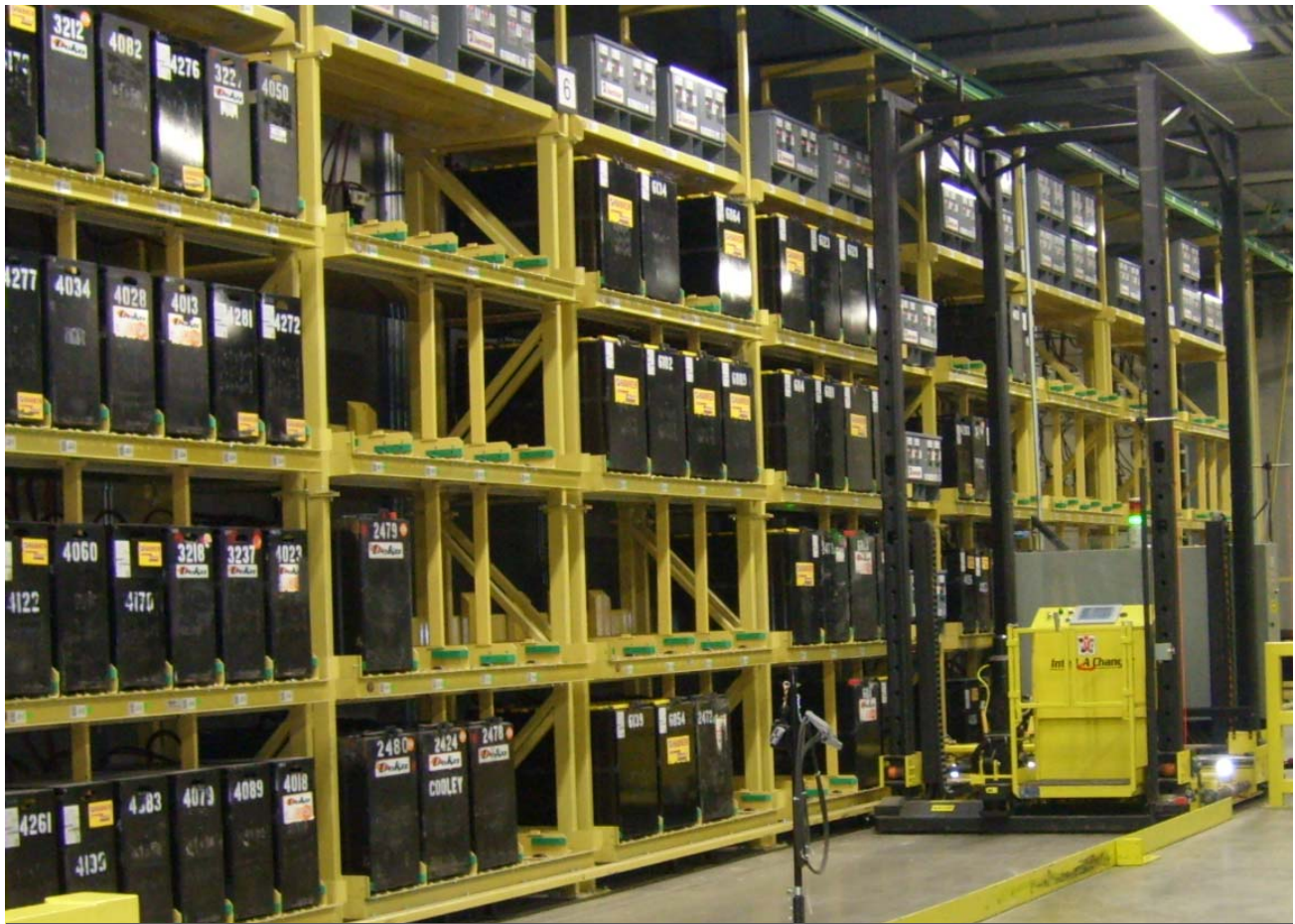
The Intell-A-Changer automatically lines up with your forklift for a perfect battery change.
